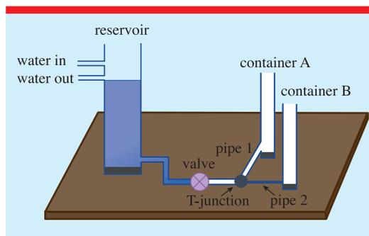
Figure 8. Schematic diagram of the apparatus.
