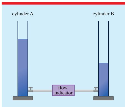
**Figure 5.** Set up with two cylinders with liquid at different levels.
