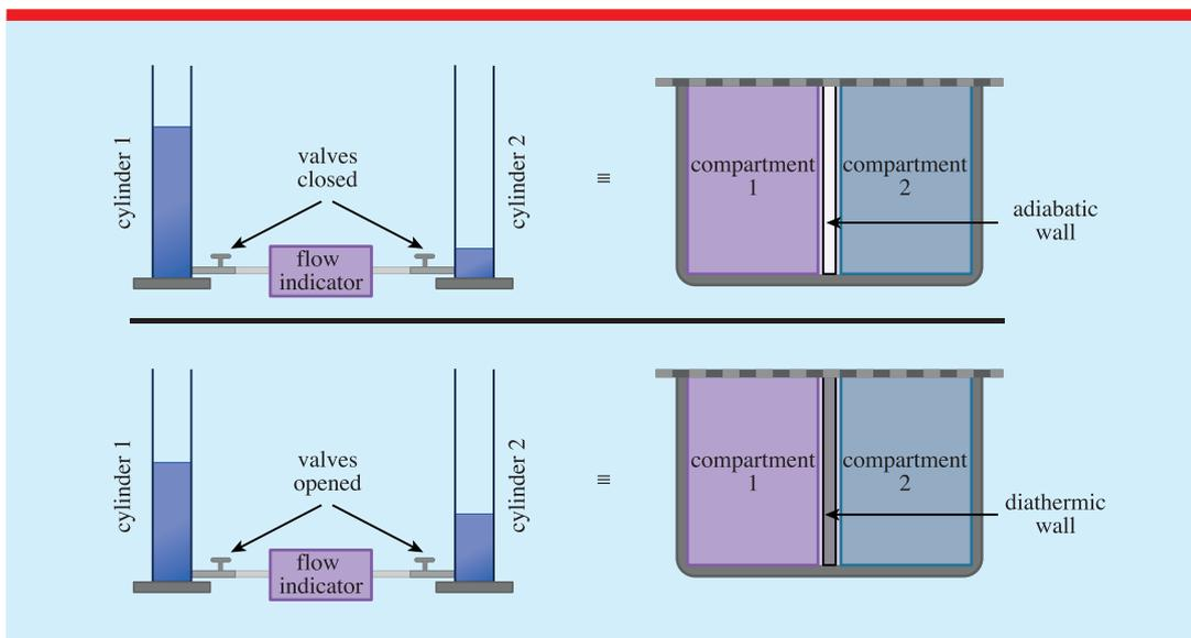
Figure 4. Analogy between liquid flow model and heat flow model of thermal equilibrium.
