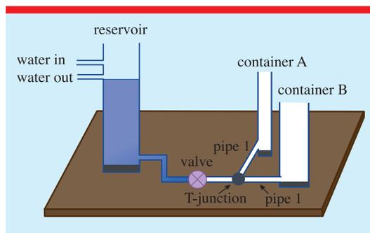
Figure 10. Schematic diagram of the apparatus.
