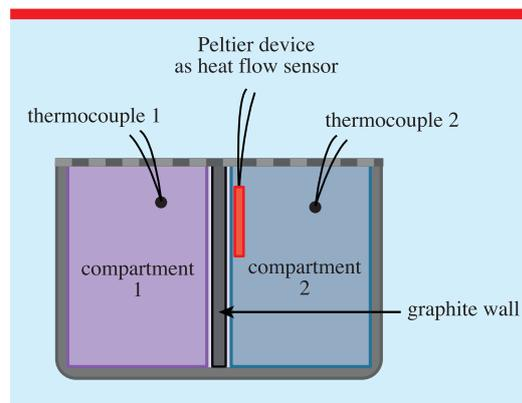
**Figure 6.** Schematic diagram of the apparatus with graphite wall in contact with both the compartments.
